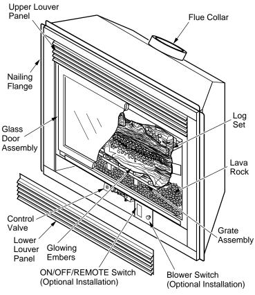
Figure 1 - Victorian Direct-Vent Fireplace with Electronic Ignition
